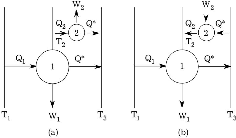
Fig. 4. Engines 1 and 2 are reversible. Reservoir 3 is basic.
