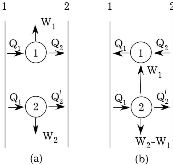
Fig. 2. Engine 1 is reversible; engine 2 may be either reversible or non-reversible.
