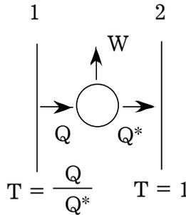
Fig. 3. Reservoir 2 is basic. Reservoir 1 is hotter than the basic reservoir.  $Q$  is the heat needing to be taken from reservoir 1 by a reversible engine to produce work  $W$  and release heat  $Q^*$  to reservoir 2.
