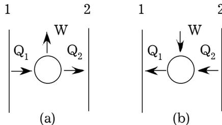
Fig. 1. Abstract heat engines. Vertical lines represent reservoirs of heat; reservoir 1 is hotter than 2. (a) Direct diagram: the engine takes heat  $Q_1$  from reservoir 1, gives heat  $Q_2$  to reservoir 2, and produces work  $W$ . (b) Reverse diagram: the engine receives work  $W$  from an external agent, takes heat  $Q_2$  from the colder reservoir, and passes heat  $Q_1$  to the hotter reservoir.
